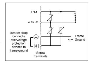
In systems with a floating neutral input (the neutral line is not referenced to Protective Earth Ground), this jumper must NOT be installed. In a floating neutral system, voltage surge protection devices such as MOVs **must** be installed from L1 to earth ground, and from L2 (Neutral) to earth ground
