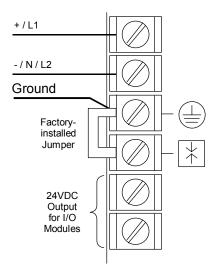
The bottom two terminals of the power supply terminal strip provide output connections to the Isolated +24 VDC. This output can be used to provide power for external circuits (within power limitations of the supply).
